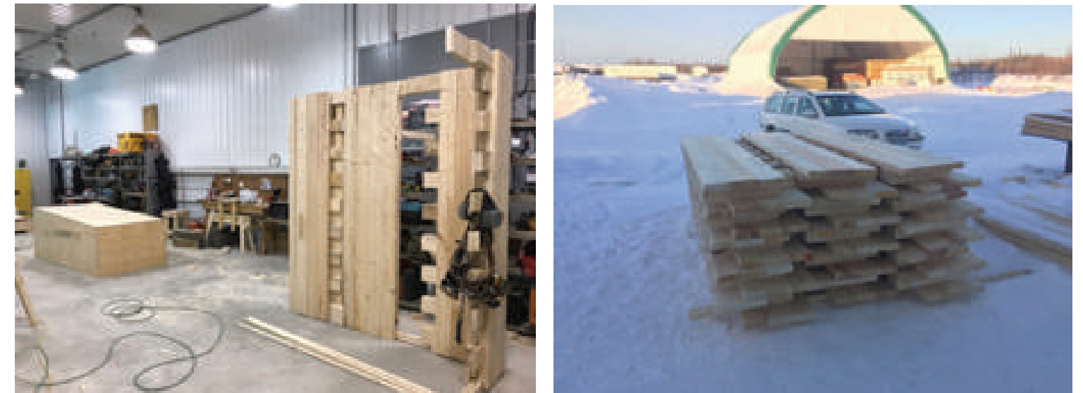
Figure 10: Cross Laminated Timber Panels design like jigsaw pieces to fit together (Heid & Tallman, 2017).
