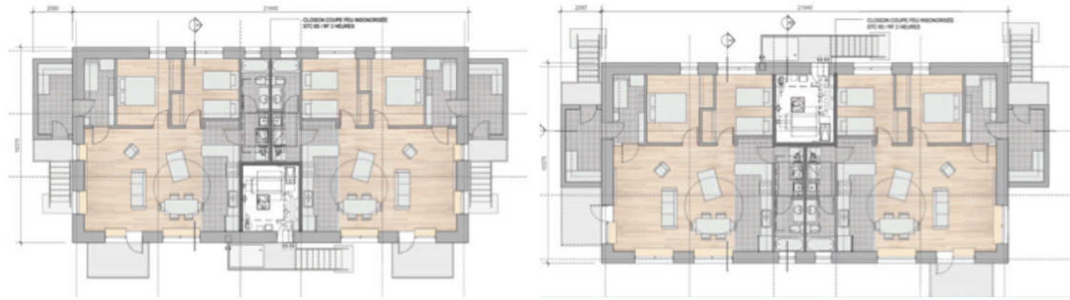
Figure 16: Duplex Floor plans – featuring living space facing south and multiple entrance options (Atkins, 2018).
