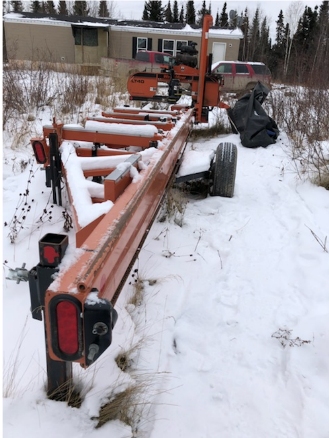
Figure 2 & 3: Existing Sawmill LT40 Portable sawmill in Garden Hill First Nation
