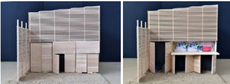
Exterior enclosures fold open and down revealing storage and creating a temporary working space.
