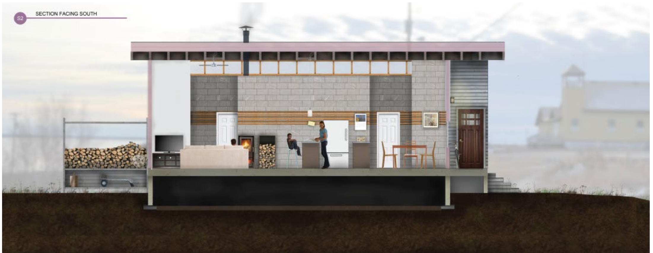
Section elevation drawing illustrating various interior and exterior spaces, activities and material finishes of the dwelling.
